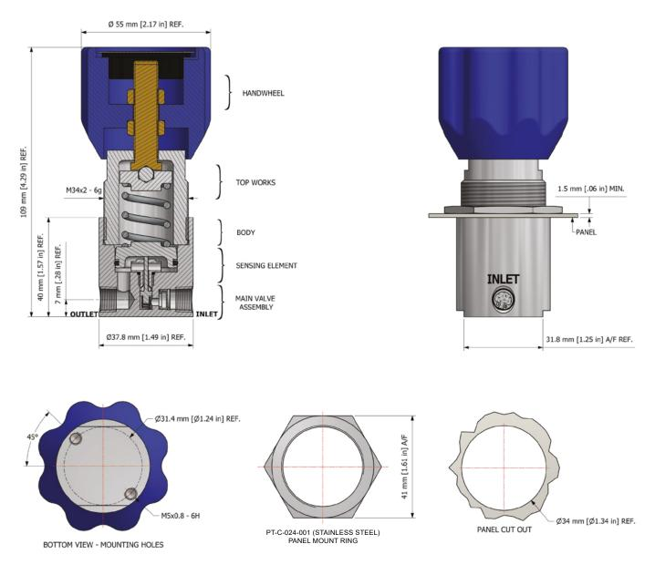
*Note:* All gauge ports are 1/8" NPT as standard Position of mounting holes may vary depending on configuration
